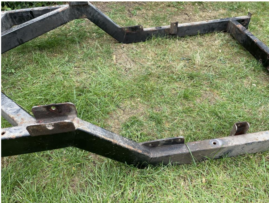
Just some of the brackets that had the sharp corners rounded off
